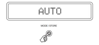
When Auto mode has been selected, press the reverse 'Skip/Scan' button to scroll down through the station frequencies or press the forward 'Skip/Scan' button to scroll up through the station frequencies.
